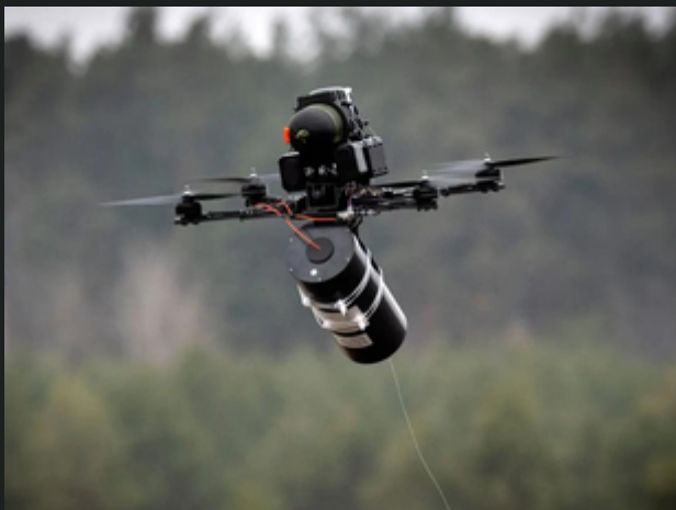
Drone with a fiber optic cable dispenser
